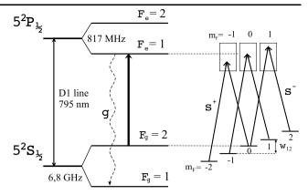
**Fig. 2** Structure of the  $D_1$  line in  ${}^{87}{\rm Rb}$  atom. The levels of the working transition  $F_g=2 \rightarrow F_e=1$  are split in the applied magnetic field into 2F+1 sublevels each. The pairs of Zeeman sublevels of the ground state  $\Delta m_F=2$  and those of excited state form a chain of three  $\Lambda$ -systems
