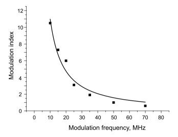
**Fig. 8** Typical dependence of the FM modulation index M of the semiconductor laser radiation vs the modulation frequency  $\Omega_{\rm mod}$ . The amplitude of the generator voltage, which creates modulation of the laser diode current, was maintained constant. Solid line shows approximation by the function  $M = A/(\Omega_{\rm mod}/(2\pi \times 1~{\rm MHz}))^B$ , where  $A = 1.7(6) \times 10^2$  and B = 1.21(14) are the approximation parameters
