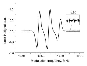
Fig. 11 Spectrum of the dark resonances taken from a vapor of Rb atoms in a buffer gas at the constant magnetic field. All resonances are split into three components due to the quadratic Zeeman effect. The magnetic field induction was roughly 14 G, the power of the pumping laser field  $P=140~\mu\text{W}$ , and the synchronous detector time constant  $\tau=3~\text{ms}$
