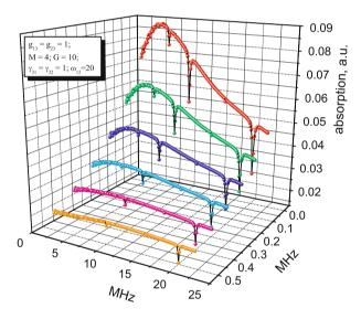
**Fig. 4** Calculated absorption spectrum of FM laser light in a cell with Rb vapor versus the modulation frequency for different decay rates  $\gamma$  from level  $5^2P_{1/2}$ , F=2 onto the level  $5^2S_{1/2}$ , F=1 equal to 0, 0.1, 0.2, 0.3, 0.4, and 0.5
